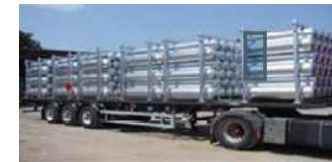
CNG Trailer (200 bar)
