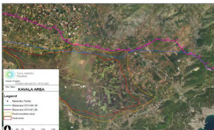
Figure.1.1: Map of the current route, illustrating the peat and transition zones from TCG Working Group (Advisory Committee) Final Deliverable Report
